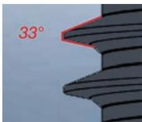
The asymmetrical flank angle of 33° guarantees much higher strength values of the formed female thread root than a common 60° thread.
