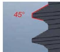
The asymmetric 45° flank angle causes smaller material displacement compared to common 60° threads and results in higher strength of the joint.
