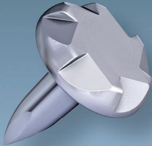
Light-weight materials can be joined to the highest strength sheets using the EJOWELD Composite Friction Fastener (CFF). This versatile and reliable joining technology allows a large variance in material thickness combinations. This progressive development has made the concept of flexible material-body a commercial reality.
