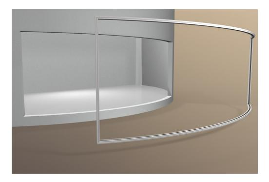
5. Apply a thick bed of silicone sealant where the bottom rail will sit
