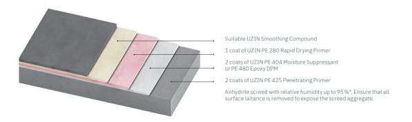
\*Up to 95 % RH for calcium sulphate screeds and suitable for under floor heating up to 90 % RH (see the product data sheets for all products).
