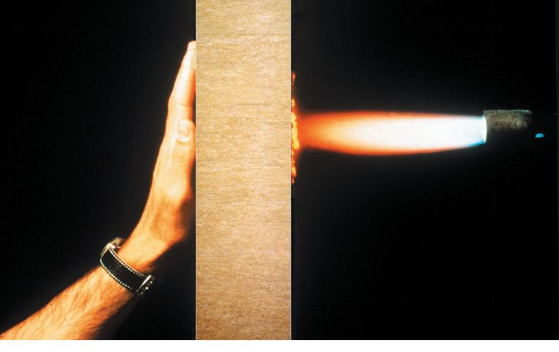
Euroclass A2-s1,d0 /According to AST® quality fire safety is composed of non-combustible panels and fire safe structures.
