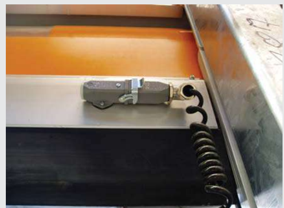
Optional: Connection of the curly cable via a Harting plug-connector
