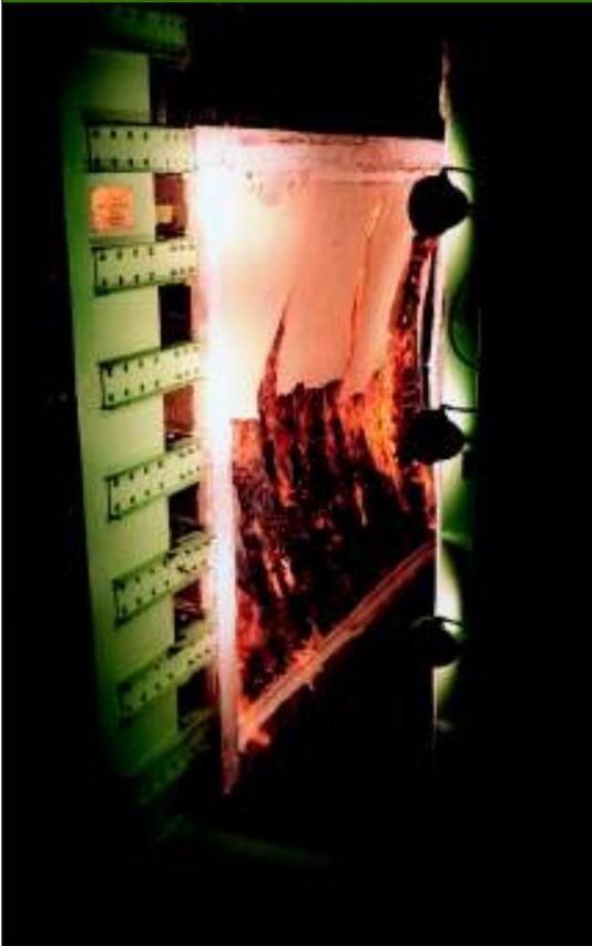
**The fire resistance rating of a structural assembly is determined by subjecting the assembly to a standard fire. The assembly, if designed to be loadbearing, must support the full design load for the duration of the fire test without allowing any flames to pass through.**
