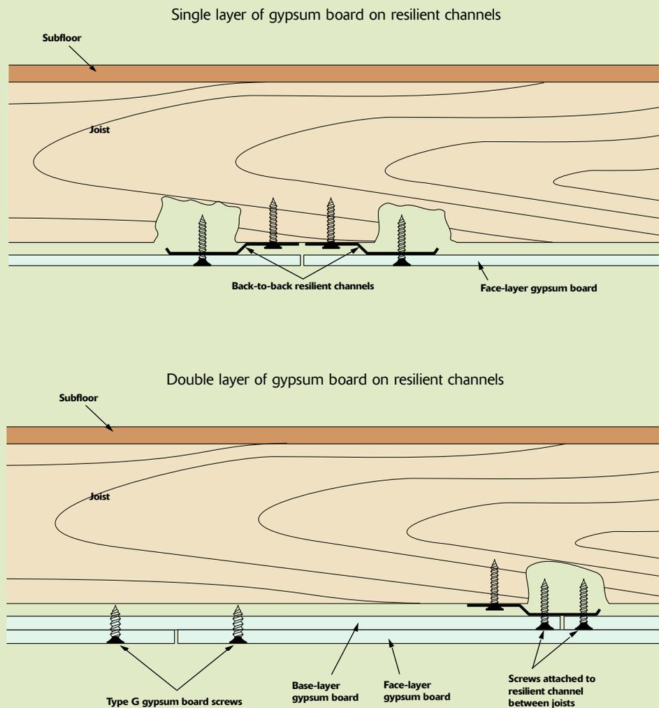
*The screws used to attach the gypsum board to resilient channels must be located away from the joists, as any direct contact with structural members would create a path for sound transmission.*
