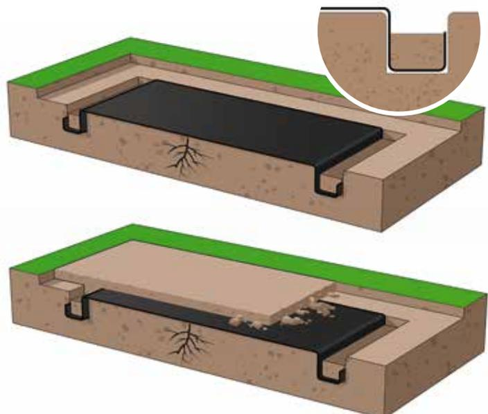
Proper use of Plantex® Platinum nonwoven fabric requires attention to the recommended installation guidelines. The product may be installed horizontally either on flat land - or on slightly sloped embankments, in which case additional considerations may be required. The joining of separate lengths should be achieved either by the DuPont recommended thermal-welding technique or by the use of Plantex® Performance Tape.
