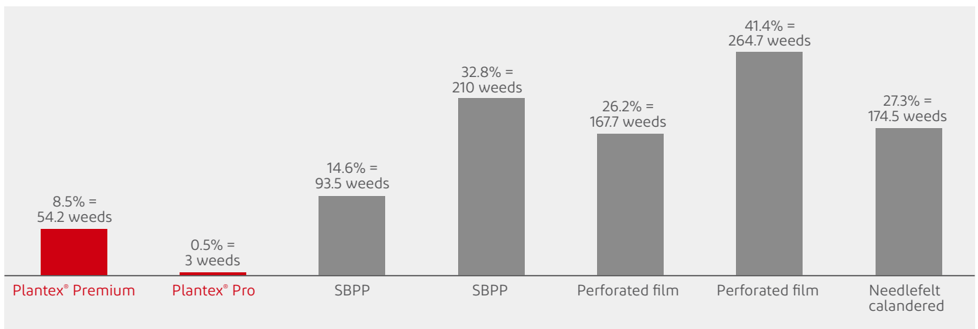
Performance expressed in % of weed growth vs. reference specimen. - Reference specimen - average count of 640 weeds
