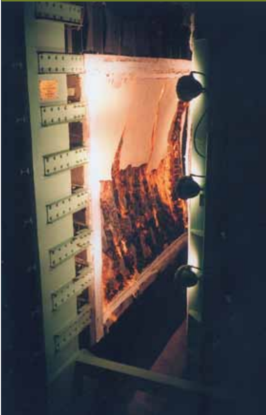
FIGURE 2: Wood-Stud Wall Assembly After 1-Hour Test
