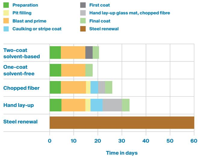
The above clearly shows at least 50% saving in time when using our chopped fiber system, compared to steel renewal. Moreover, the material and application of our chopped fiber system is cheaper, resulting in further cost savings for tank farm operators.
