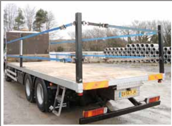
Six wheeler rigid flatbed with Side Rail Fall Protection
