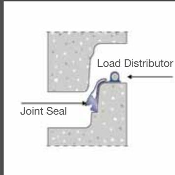
Seal references are Forsheda F-171 or DS SDVSEAL, manufactured to BS EN 681-1 type WC. Actual size is dependent on manhole diameter.
