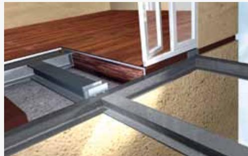
Steel-to-steel connection: Isokorb® Type KST.
