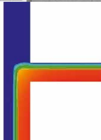
Heat flow lines and temperature distribution of Schöck Isokorb® Type AXT provide an efficient solution and minimize the thermal bridge where it occurs.
