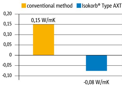
High psi-values for conventional methods result in high energy loss and increased energy costs. While negative psi-values for the Isokorb® Type AXT provide a positive input for your energy balance.
