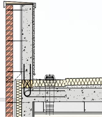
Efficient solution with Schöck Isokorb® Type AXT.
