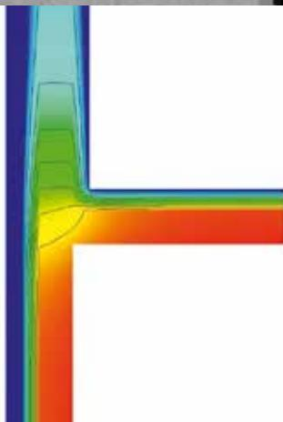
Heat flow lines and temperature distribution of conventional methods show that the parapet will be heated and therefore requires additional energy.
