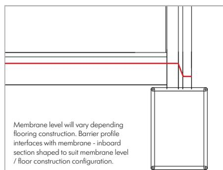
Membrane level will vary depending flooring construction. Barrier profile interfaces with membrane - inboard section shaped to suit membrane level / floor construction configuration.
