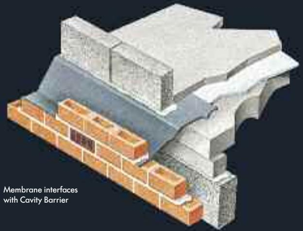
Membrane interfaces with Cavity Barrier
