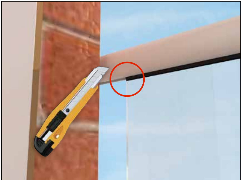
15. Trim off excess rubber.
