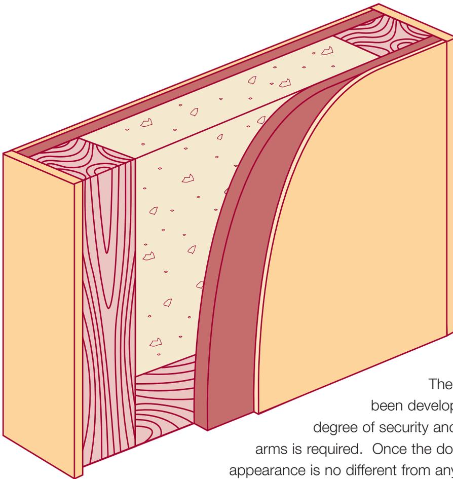
The Noberne Bullet Resisting door has been developed for use in areas where a high degree of security and resistance to the discharge of fire arms is required. Once the door is fixed in position its appearance is no different from any other flush door. The door has been tested in accordance with British Standard 5051 Part 1 1973 with the following successful results.
