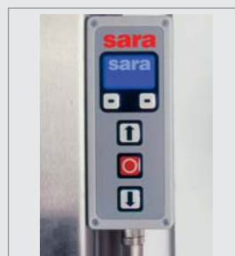
Display unit in a small box placed at the side frame.
