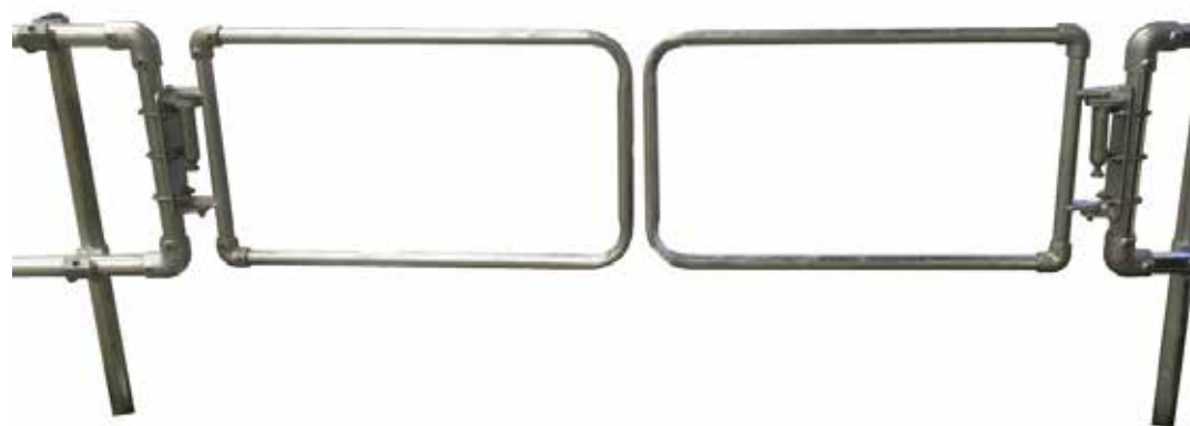
M. Using a 24mm socket & spanner tighten the bolt until the gate completely closes. (You may have to hold the socket whilst using the ratchet). Once the gate is completely closed tighten the locking nut to hold the tension. Caution:- Hold ratchet firmly and do not release until the lock nut is tightened. Repeat as necessary to ensure that the gate closes sufficiently.
