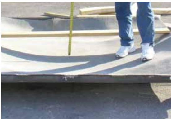
**Image: The *PITT-CHAR XP* coating intact after 4-bar overpressure blast test**
