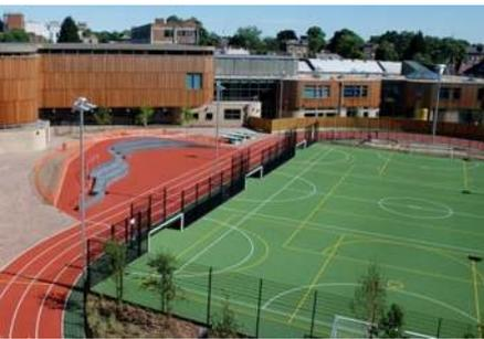
Posts and panels are galvanised to protect against corrosion and have a tough, low-maintenance polyester powder coat applied to provide an attractive aesthetic finish. This coating is available in a choice of standard colours, or custom colours can be applied to special order. If football is to be played, goal recesses can be incorporated within the fence.
