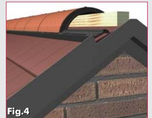
Trim each undercloak dry verge at the ridge ensuring there is a least a 5mm gap where the two undercloak dry verge sections meet. This gap is necessary to allow for expansion caused by the heat of the sun.
