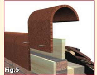
6. Lay subsequent mono-ridge tiles and top fillers positioning a ridge to ridge seal between each mono-ridge as you proceed.
