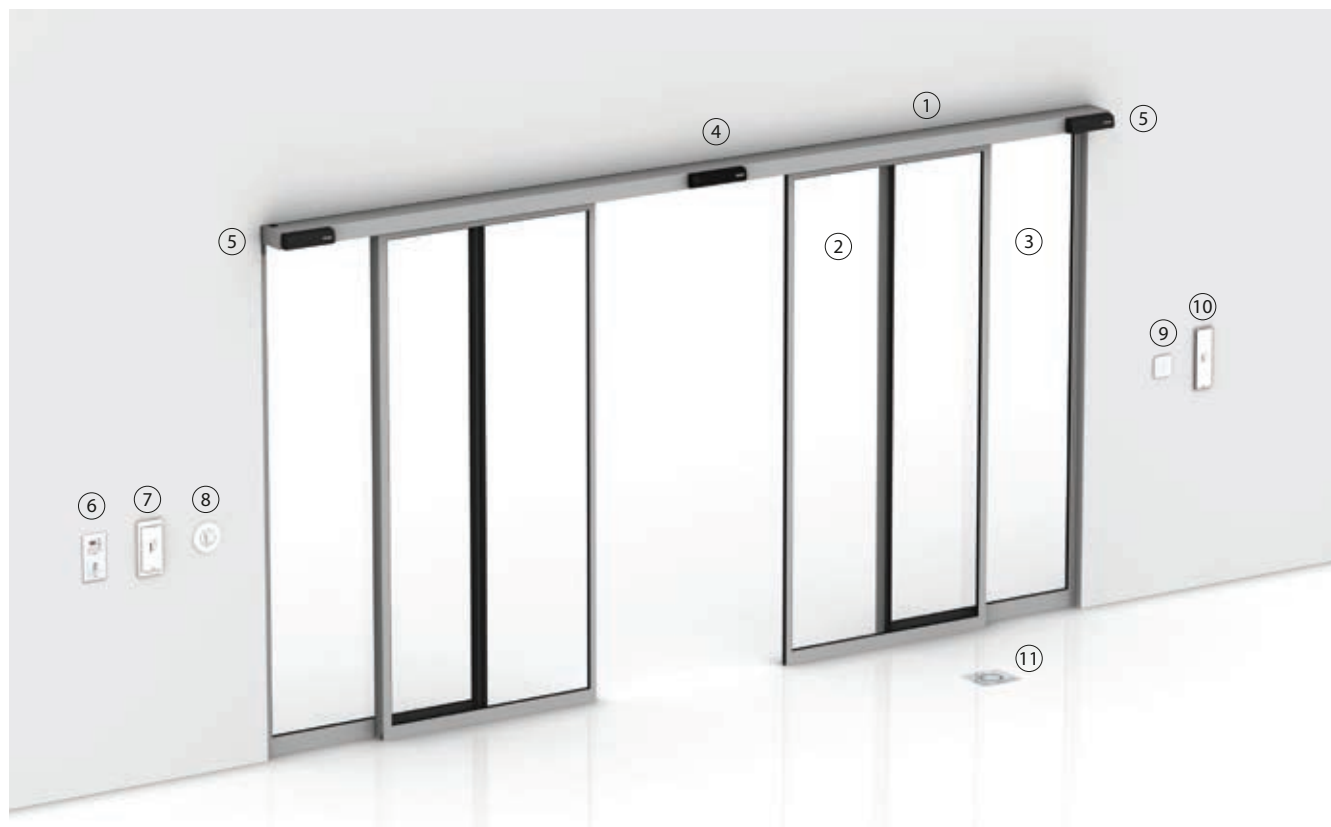
1 = Sliding door drive | 2 = Moving leaf | 3 = Side panel | 4 = Combined detector | 5 = Active infrared detector | 6 = Programme switch with key switch | 7 = Plastic elbow switch | 8 = LED sensor switch glass | 9 = Non-contact proximity switch | 10 = Elbow switch | 11 = LED sensor foot switch
