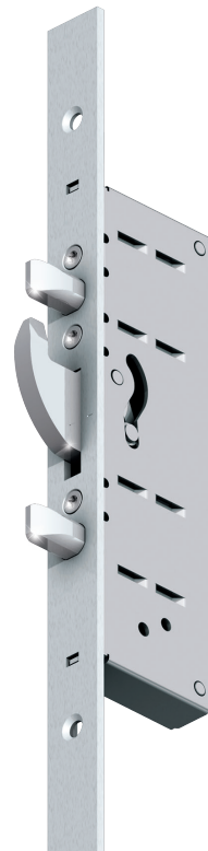
Type 11 locks: key or handle operated 3-point lock with central day & deadbolt latch as well as hook and dual-round bolt on top and bottom for enhanced safety.
