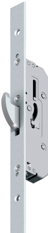
Type 3 locks: key or handle operated 3-point lock with central day & deadbolt latch as well as hook bolt on top & bottom for high safety.
