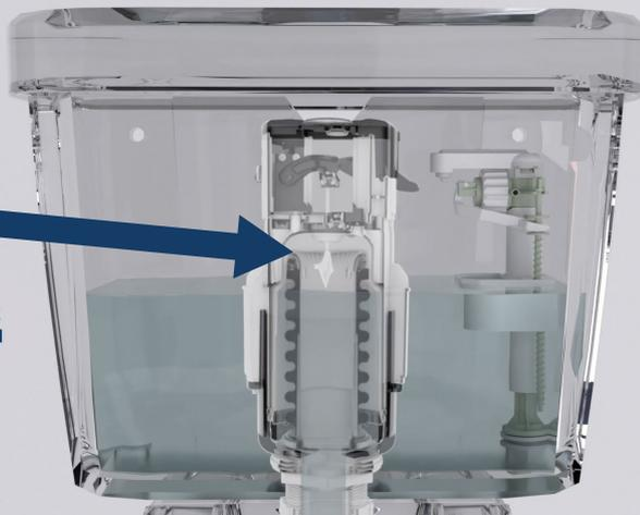
The multi-award winning Easyflush<sup>EVO</sup> will not leak due to debris, scale, or degradation of the seal, as it has been designed without a flush seal below the water line, unlike traditional WC flush drop valves.
