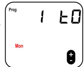
**Step 5:** Press the TIME button to copy the programs. The 'TO' will flash to confirm the programs have been copied.
