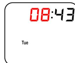
**Step 3:** Press the TIME button. The day will flash. Use the + and - buttons to change the day. Once set, press the TIME button to return to the main screen.
