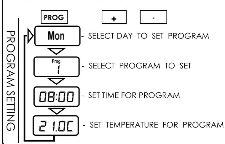
This section provides an example of how to set the 7-day program for one day. The example will program the timer to maintain 21°C from 08:00 until 16:00. It will maintain 4°C from 16:00 onwards. It does this by setting the programs as follows;
