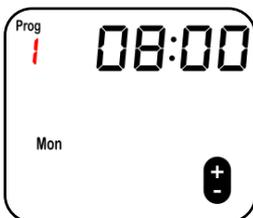
**Step 3:** Press the PROG button. The time should flash. Use the + and - buttons to set the time you want the heating to switch on.
