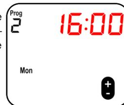
**Step 8:** Press the PROG button. The temperature should flash. Use the + and - buttons to select a frost protection temperature.
