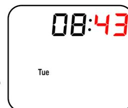
**Step 2:** Press the TIME button. The hours will flash. Use the + and - buttons to adjust the hours.
