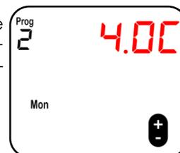
**Step 9:** Repeat these steps for programs 3-6 if additional time periods are required. Any programs not being utilized must be deactivated. To do this, simply select the program in question as per step 6 and press the TIME button. The time should change to dashes as shown below. To reactivate the program, simply press the TIME button again.
