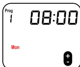
**Step 2:** Press and hold TIME for 5 seconds to enter the copy day setting.
