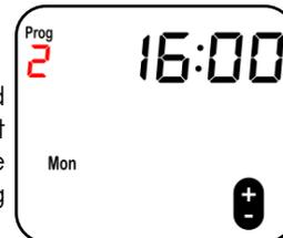
**Step 7:** Press the PROG button. The time should flash. Use the + and - buttons to select the time you want the heating to switch off.
