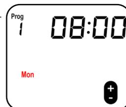
**Step 6:** Press the PROG button. Prog 1 in the top left of the display should flash. Use the + button to increment this to Prog 2. (Note: you can cycle between the different programs using the + and - buttons)
