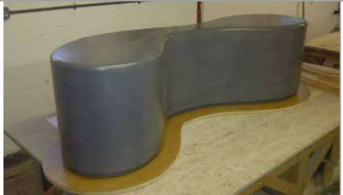
Positive-form master used for creating mould for Marlborough bench
