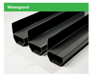
The Wykamol Waterguard Drainage Channel is a PVC drainage conduit for the control of water ingress in below-ground waterproofing situations. Wykamol Waterguard has a flange up-stand and is fitted around the perimeter of the floor at the vulnerable wall to floor junctions, directing any ingress of water towards a sump chamber or drain.
