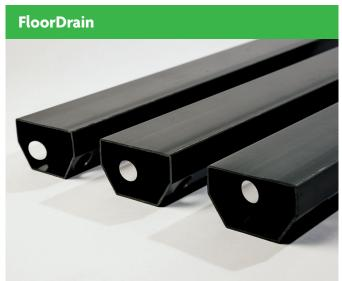
The Wykamol Floor Drain Channel is a PVC drainage conduit for the control of water ingress in below-ground waterproofing situations. Wykamol Floor Drain is flangeless (no up-stand) and can be fitted across the centre of the basement floor, directing any ingress of water towards a sump chamber or drain.
