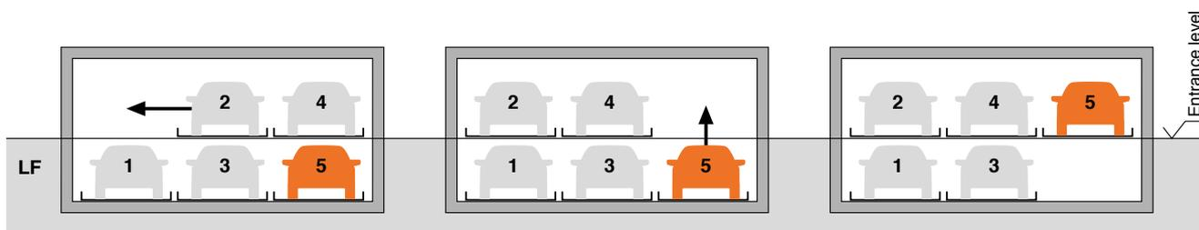
For driving the vehicle off platform No. 5 the ground floor parking platforms are shifted to the left
