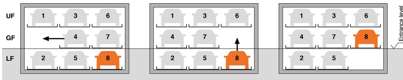
For driving the vehicle off platform No. 8 the ground floor parking platforms are shifted to the left
