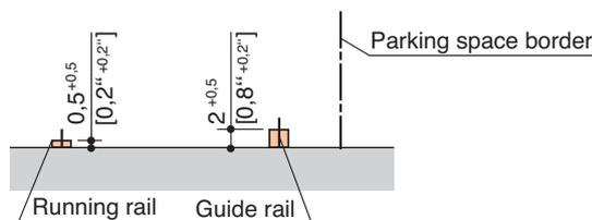
**!** Projection of the guide rail above top edge of finished floor is mandatory on both sides of the rail including the level for the drive!
