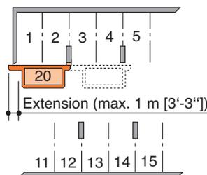
When using **Drive D**, no one-sided ParkBoard extensions are necessary.
