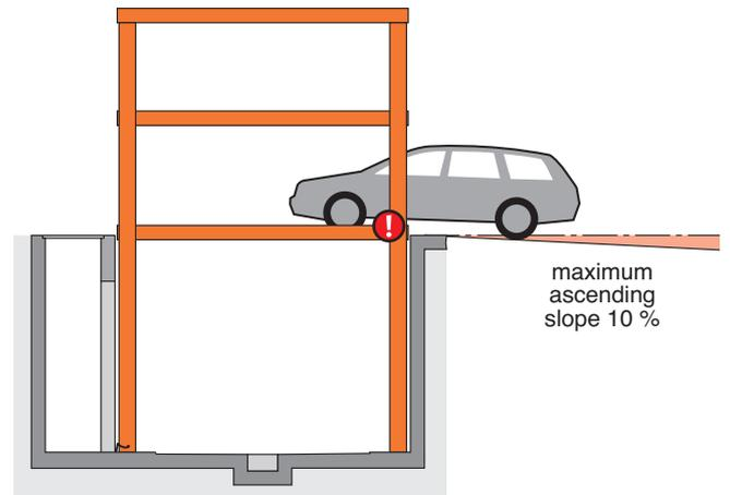
**!** The illustrated maximum approach angles must not be exceeded. Incorrect approach angles will cause serious manoeuvring & positioning problems on the parking system for which the local agency of KLAUS Multiparking accepts no responsibility.
