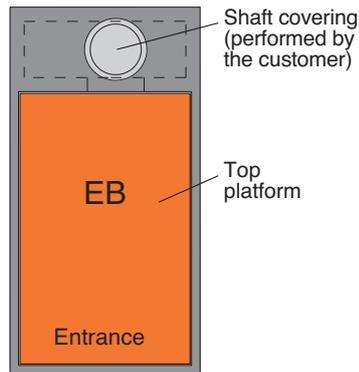
Serial system (with dividing walls)
