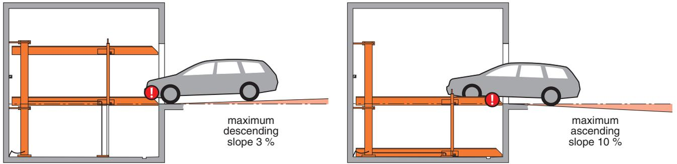
**!** The illustrated maximum approach angles must not be exceeded. Incorrect approach angles will cause serious manoeuvring & positioning problems on the parking system for which the local agency of KLAUS Multiparking accepts no responsibility.
