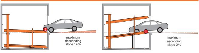
The illustrated maximum approach angles must not be exceeded. Incorrect approach angles will cause serious maneouvring & positioning problems on the parking system for which the local agency of KLAUS Multiparking accepts no responsibility.
