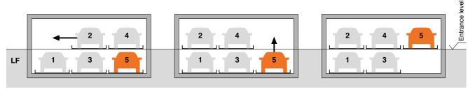
For driving the vehicle off platform No. 5 the ground floor parking platforms are shifted to the left The empty space is now below the vehicle which shall be driven off the platform. The platform No. 5 will be lowered.
