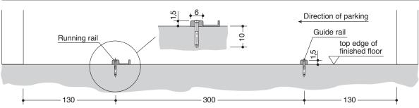
Tolerances for the evenness of the carriageway must be strictly complied with in accordance with DIN (= German Industrial Standard) No. 18202, chart 3, line 3. No expansion joints are permitted within the area of the rail system.
