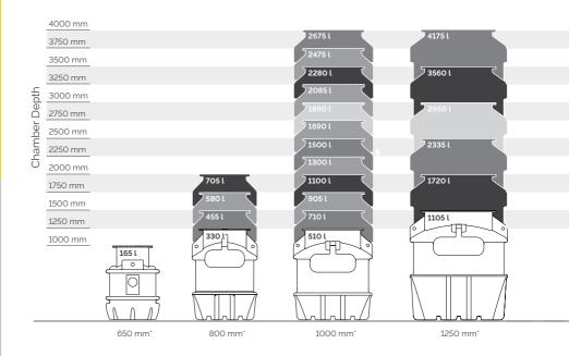
Capacities shown are for highest possible inlet invert. Please contact us for fabrication sheets detailing chamber dimensions and capacities for varying inlet depths.
