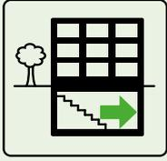
In a repair situation, the basement can be waterproofed from the inside without excavating the soil around the building. This means that the basement is permanently waterproofed without the necessity of doing any sort of earthwork. This type of waterproofing is possible with the KÖSTER systems even when the wall has active leakages.
