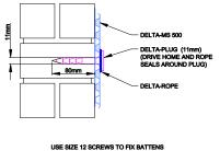
USE SIZE 12 SCREWS TO FIX BATTENS OR METAL LINING SYSTEMS USE 11mm DRILL BIT
