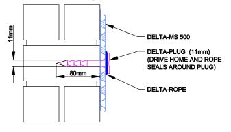
USE SIZE 12 SCREWS TO FIX BATTENS OR METAL LINING SYSTEMS USE 11mm DRILL BIT
