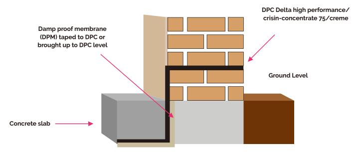
\*DPC installed 150mm fom external ground level
