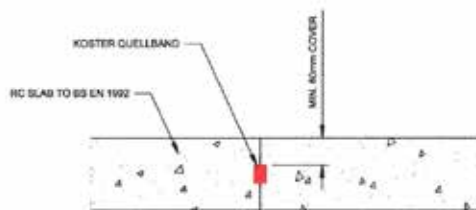
NEW SLAB CONSTRUCTION JOINT
