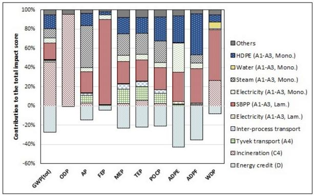
For most of the impact categories, more than 70 % of the impact is dominated by the functional layer (HDPE granulates and steam supply mainly) and lamination (SBPP supply mainly) production steps; except for **ODP** which is dominated by the incineration of the product after its use.
