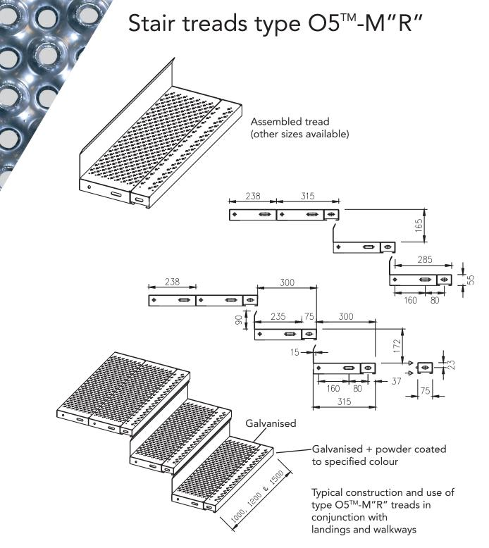
Stair tread type O5<sup>™</sup>-M"R" is based on the fabricated O5 M tread. Identified by 5 mm dia. punched and drainage holes is predominantly used in public areas and high working platforms.
