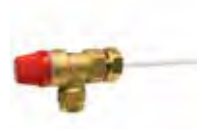
Temperature & pressure relief valve* 3/4" BSP union nut x 15mm (10 bar / 90°C)
