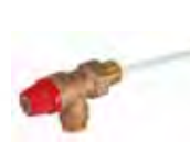
Temperature & pressure relief valve* ½"NPT x 15mm (7 bar / 90°C)
