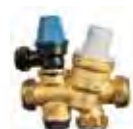
Inlet control set with balanced cold (3 bar PRV, 6 bar expansion relief)
