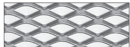
LD16 (Fe) (Scale 1:1) Open area: 47% Weight: 4.0 kg/m 2 Thickness: 3.0 mm Dimensions: 16 x 8.0 - 2.0 x 1.0
