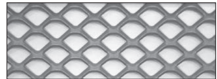
LS10 (Fe) (Scale 1:1) Open area: 57% Weight: 3.2 kg/m 2 Thickness: 2.0 mm Dimensions: 10 x 7.0 - 1.5 x 1.0
