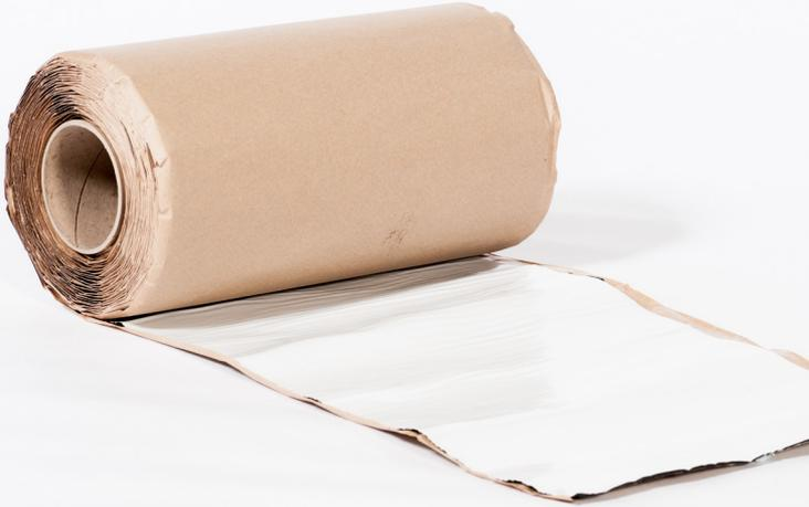
The Cordek Gas Resistant Detailing Strip is used for detailing work, when sealing a sheet membrane to penetrations e.g. steel columns, manholes, piles etc. It is manufactured using aluminium /polythene laminate coated on one surface, with an additional layer of self-adhesive polymer modified bitumen.
