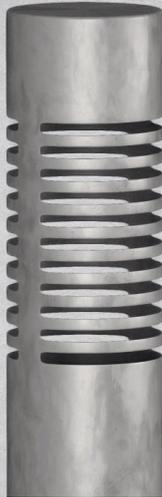
The Cordek Gas Vent Bollards provide an efficient and economical method of venting ground gases from beneath a building to the atmosphere when connected to a suitable venting system e.g. Cordek Ventform or Cellvent. Vent Bollards are usually installed in locations where alternative venting methods, such as air bricks, cannot be used or where a vent with a high level of free air flow is required.
