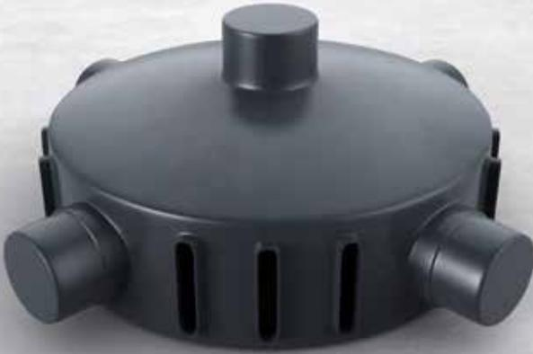
A Cordek Radon Sump acts as an extraction point for radon gases beneath buildings within radon affected areas. If a radon sump is positioned within a permeable granular layer beneath a ground floor slab and subsequently connected to an extract fan then the penetration of hazardous radon gas into the building is minimised. Cordek also provide a range of additional components including membranes, DPC's and vent outlets to provide a solution to the issues posed by radon gas to new constructions.
